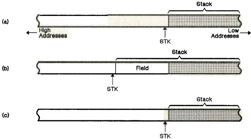
Figure 3-7. Auxiliary Stack Grows toward Higher Addresses
