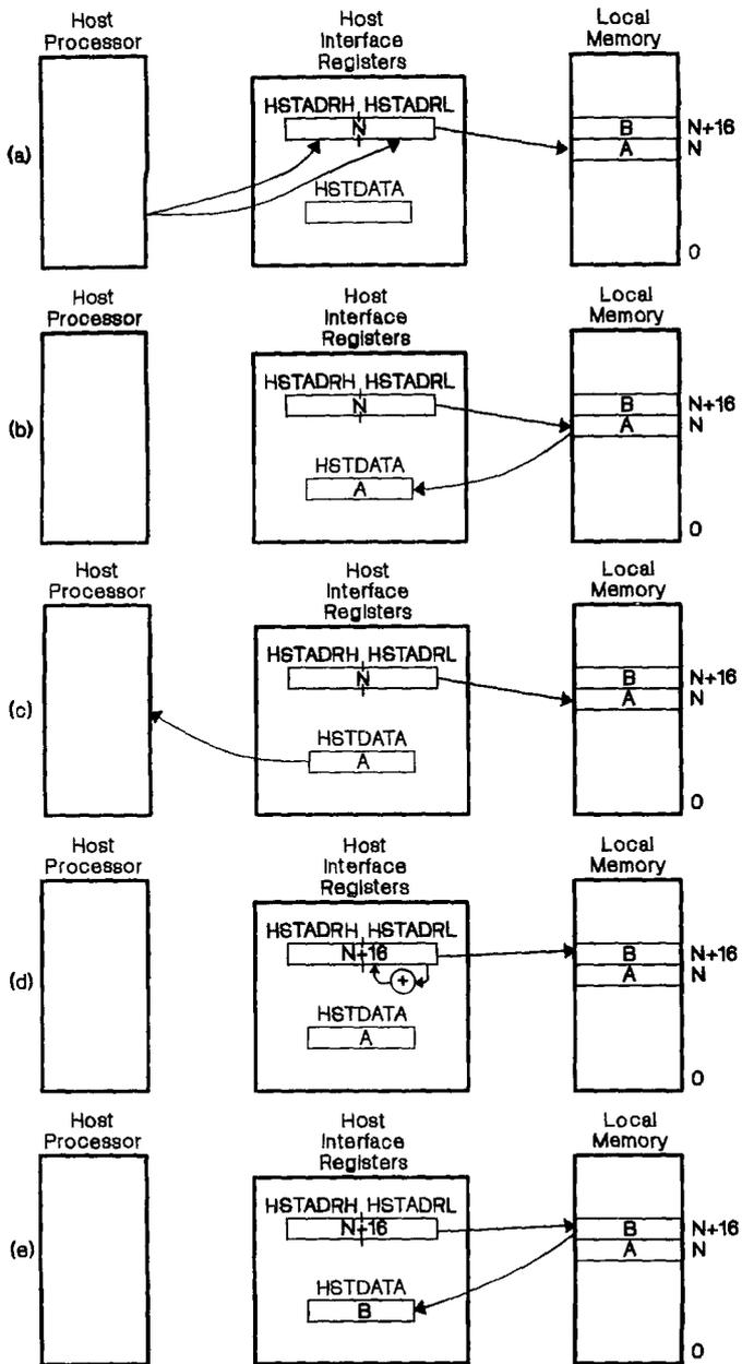
Figure 10-10. Host Indirect Read from Local Memory (INCR=1)
