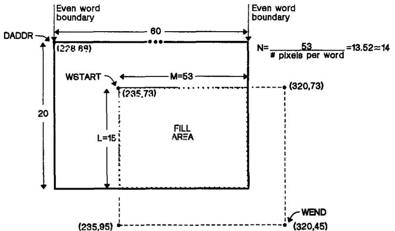
Figure 13-5. FILL XY Timing Example
