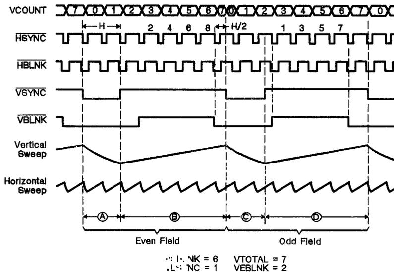
Figure 9-10. Interlaced Video Timing Waveform Example
