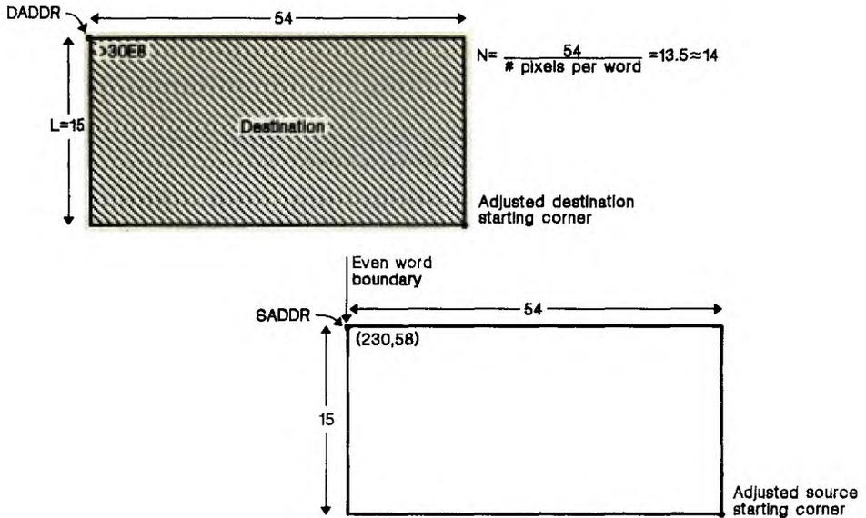
Figure 13-9. PIXBLT XY,L Timing Example
