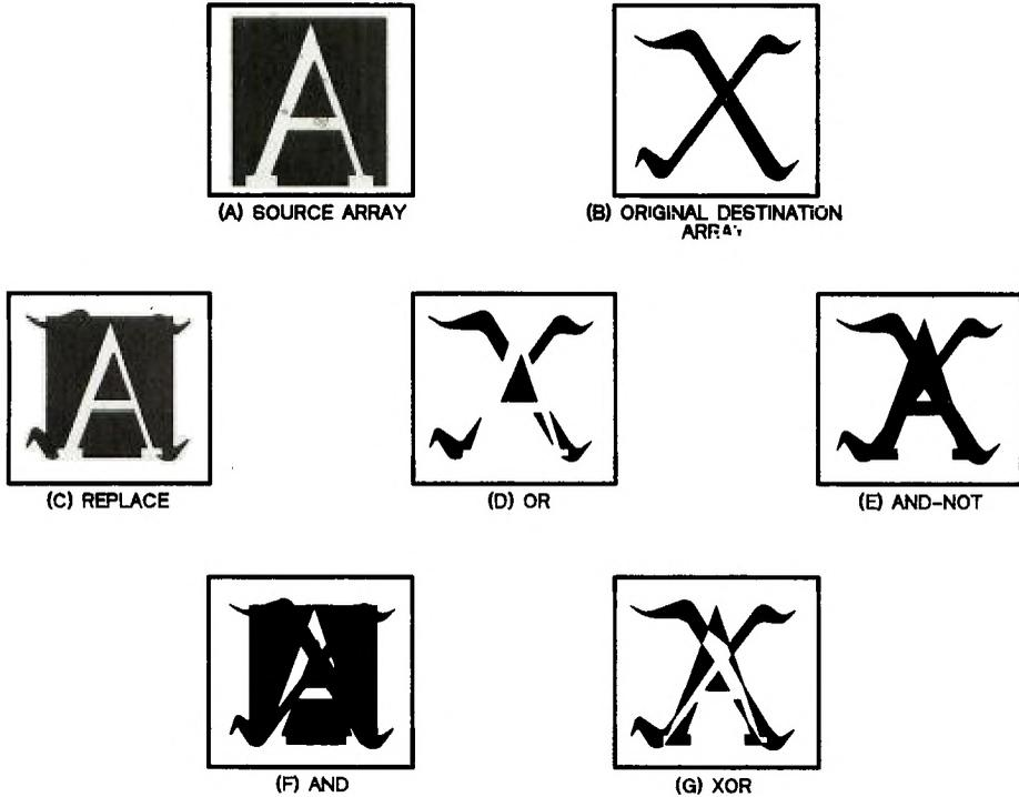
Figure 7-7. Examples of Operations on Single-Bit Pixels
