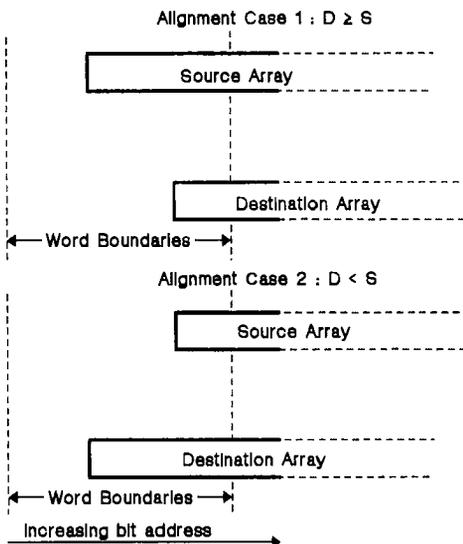
Figure 13-8. Source to Destination Alignments
