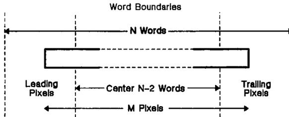
Figure 13-10. Pixel Block Alignment in X
