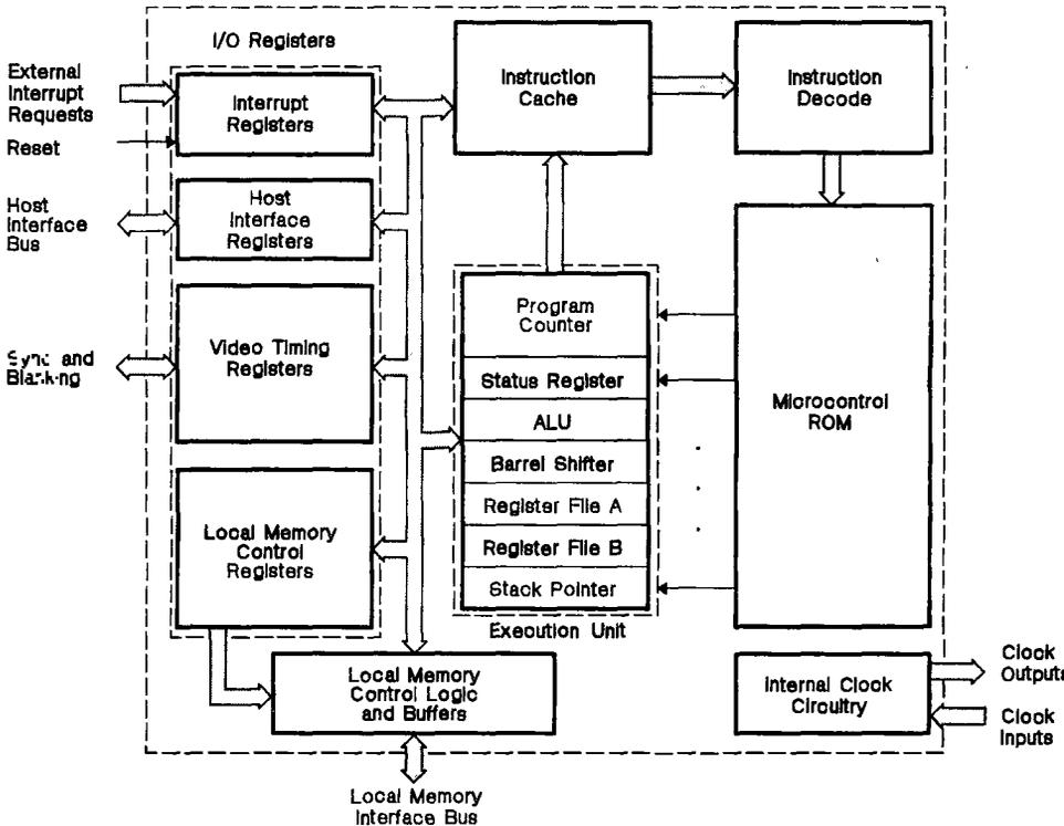
Figure 1-2. Internal Architecture Block Diagram
