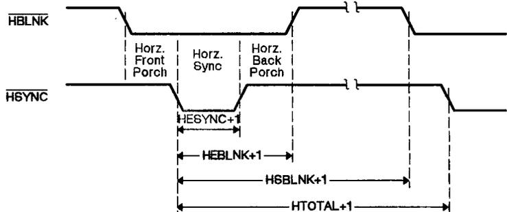
Figure 9-2. Horizontal Timing
