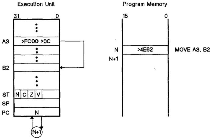
Figure 12-3. Register Direct Addressing Mode
