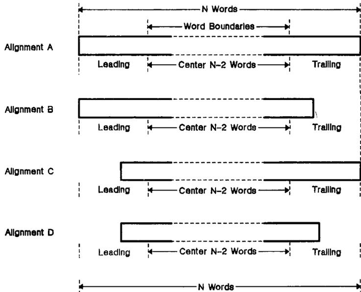
Figure 13-11. Pixel Block Row Alignments
