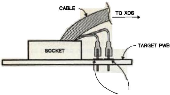
PLACE FEMALE CONNECTOR FROM XDS TARGET CABLE ASSEMBLY OVER MALE CONNECTOR STAFF ON PWB, WHICH ARE CONNECTED TO THE GROUND OF THE TARGET SYSTEM
