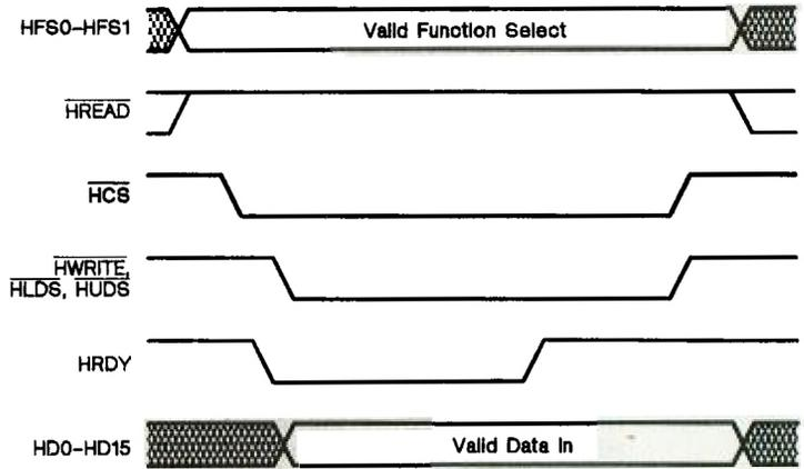
Figure 10-8. Host Interface Timing - Write Cycle With Wait
