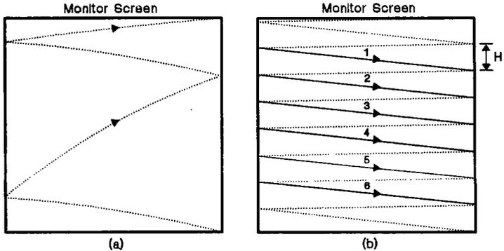
Figure 9-7. Electron Beam Pattern for Noninterlaced Video
