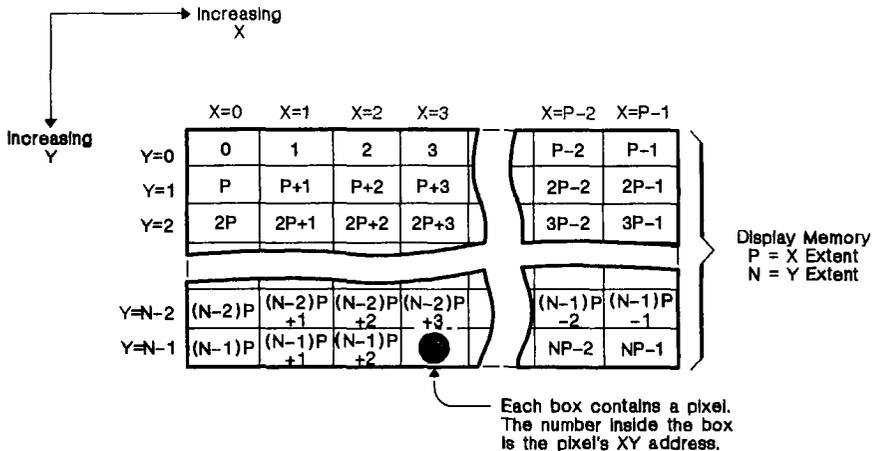
$$\begin{aligned} \text{Display Pitch} &= (\text{X extent}) \times (\text{pixel size}) \\ &= \text{Differences in 32-bit memory addresses} \\ &\quad \text{of two vertically adjacent pixels} \end{aligned}$$
