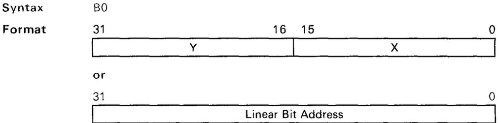
**Description** SADDR contains the source array address pointer for PIXBLTs. Generally, SADDR points to the pixel with the lowest address in the source array. When a corner adjust is necessary, the GSP automatically adjusts SADDR to point to the selected starting corner of the source array. (For PIXBLT L,L, however, you must manually adjust SADDR to point to the starting corner. This feature allows you to use PIXBLT L,L for manipulating pixel arrays with pitches that are not powers of two.)
