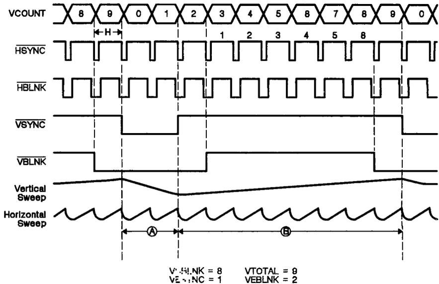
Figure 9-8. Noninterlaced Video Timing Waveform Example
