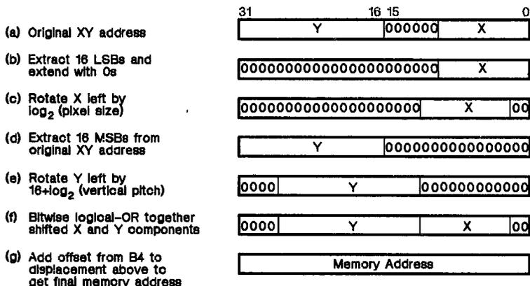
**Figure 4-11. Conversion from XY Coordinates to Memory Address**
