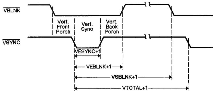
Figure 9-5. Vertical Timing for Noninterlaced Display
