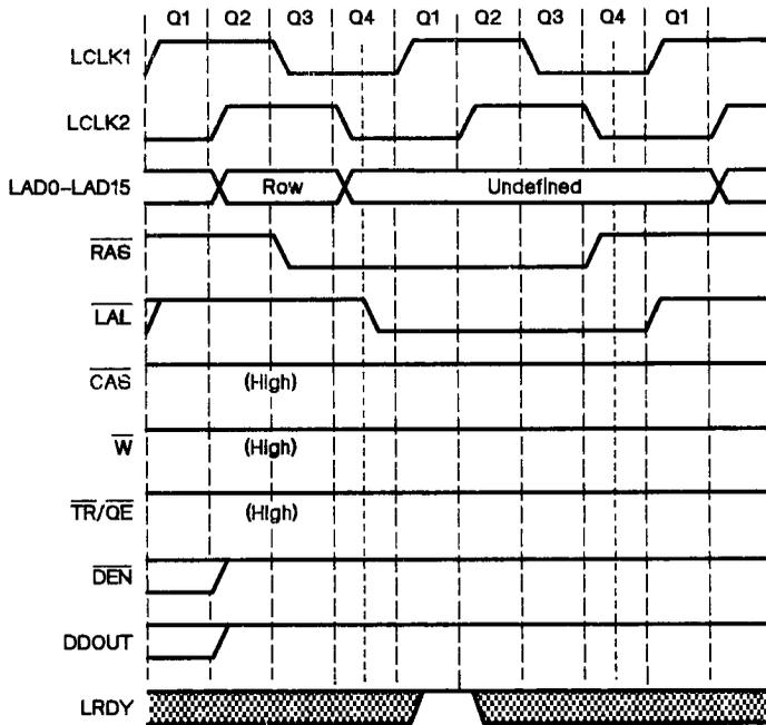
Figure 11-7. Local Bus  $\overline{\text{RAS}}$ -Only DRAM-Refresh Cycle Timing
