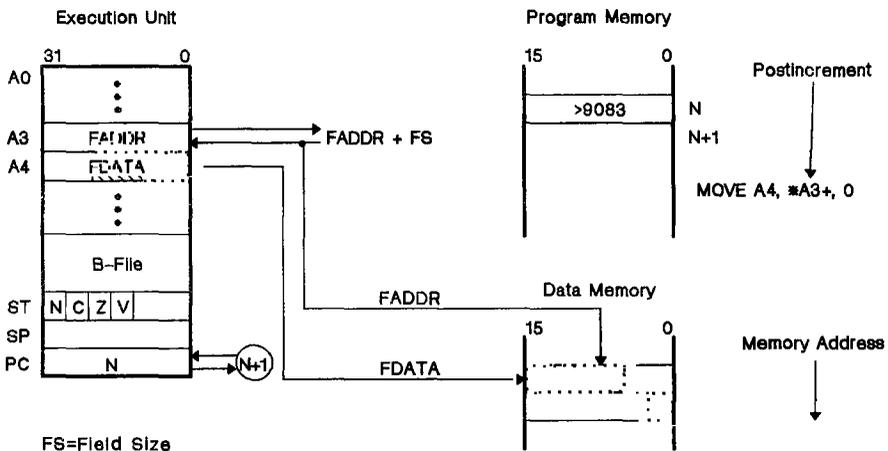
Figure 12-7. Register Indirect with Postincrement Addressing Mode
