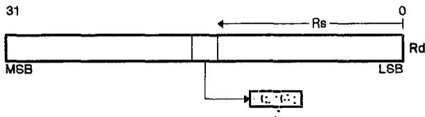
**Description** BTST tests the specified destination register bit and sets status bit Z accordingly. The five LSBs of the source register specify the bit to be tested (the 27 MSBs are ignored).
