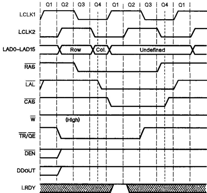
Figure 11-6. Local Bus Memory to Shift Register Cycle Timing
