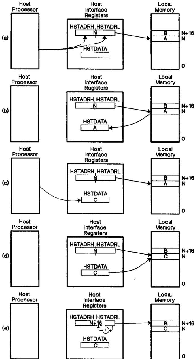
Figure 10-11. Host Indirect Write to Local Memory (INCW=1)
