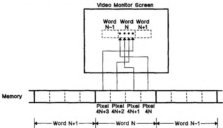
Figure 4-5. Mapping of Pixels to Monitor Screen
