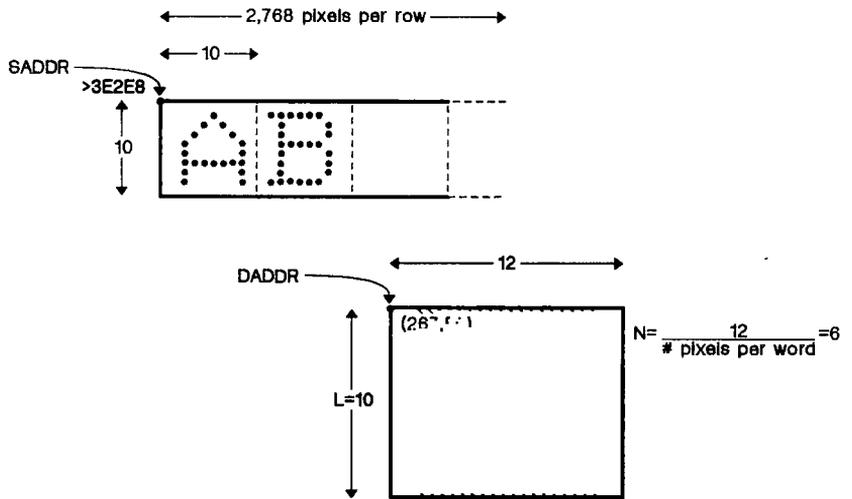
Figure 13-12. PIXBLT B,XY Timing Example
