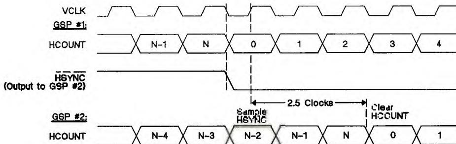
**Figure 9-11. External Sync Timing - Two GSP Chips**
