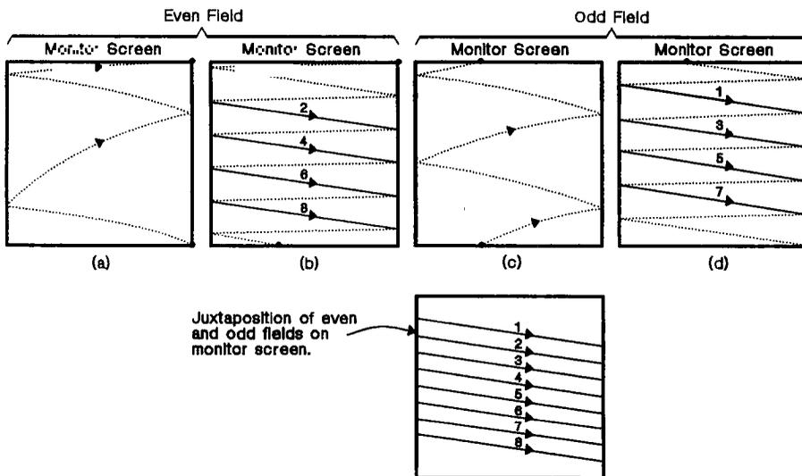
Figure 9-9. Electron Beam Pattern for Interlaced Video
