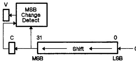
The left shift count is contained in the 5-bit K field of the instruction word. The assembler accepts only absolute expressions as valid K operand values. SLA executes slower than SLL because overflow detection. If the value specified is greater than 31, the assembler issues a warning and sets the value of the K field equal to the five LSBs of the K operand value specified.
