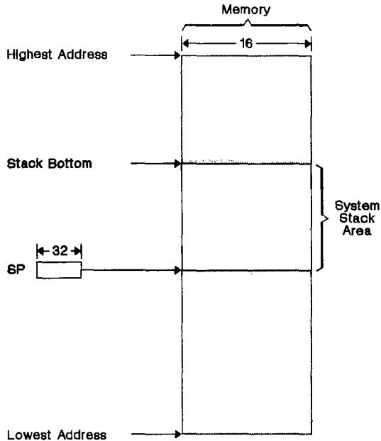
Figure 3-4. System Stack
