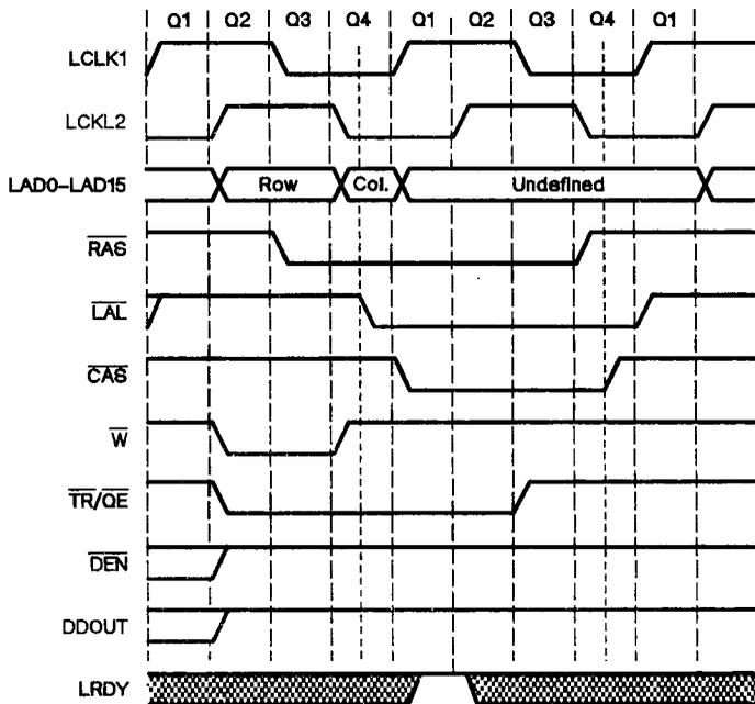
Figure 11-5. Local Bus Shift Register to Memory Cycle Timing
