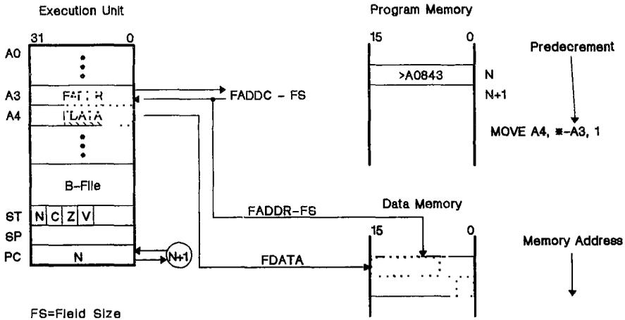
Figure 12-6. Register Indirect with Predecrement Addressing Mode
