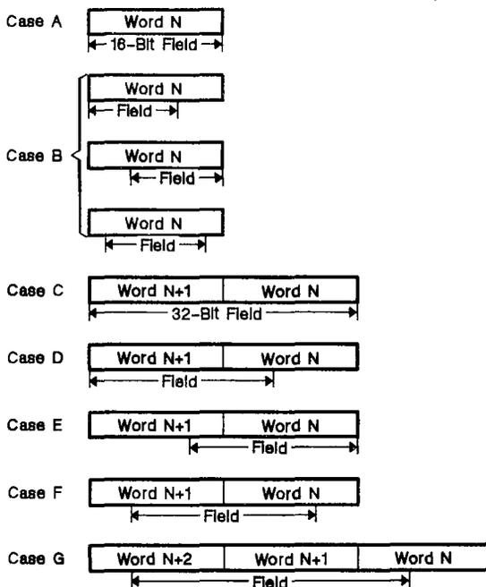
Figure 13-1. Field Alignments in Memory
