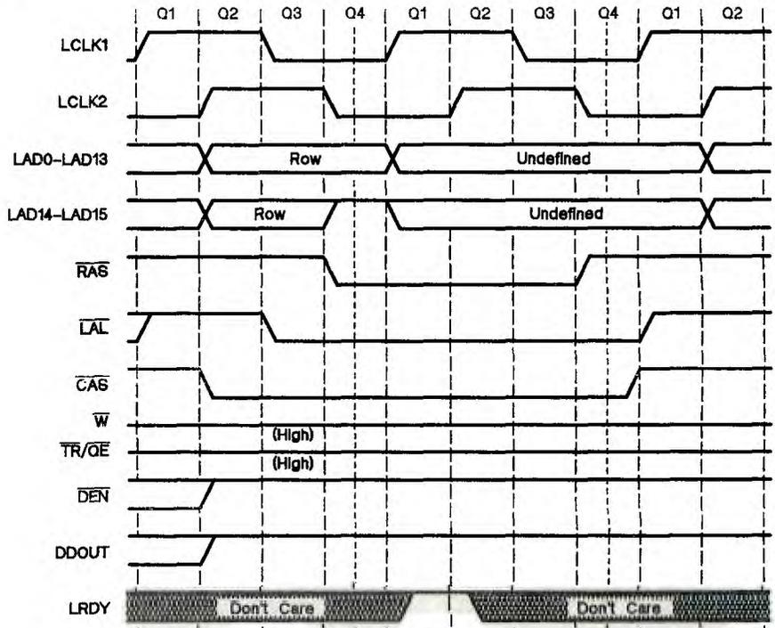
Figure 11-8. Local Bus  $\overline{\text{CAS}}$ -Before- $\overline{\text{RAS}}$  DRAM-Refresh Cycle Timing
