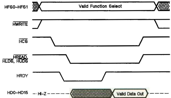
Figure 10-9. Host Interface Timing - Read Cycle With Wait
