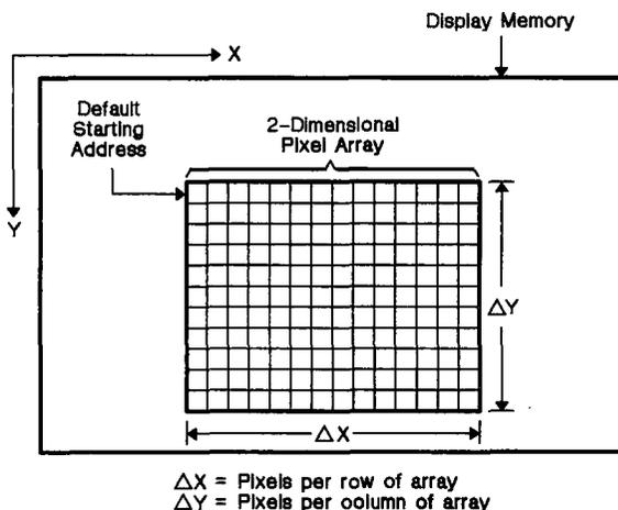
Figure 4-12. Pixel Array
