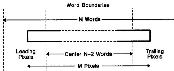
**Figure 13-6. Pixel Block Alignment in X**
