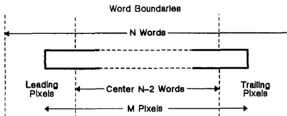
**Figure 13-3. Pixel Block Alignment in X**
