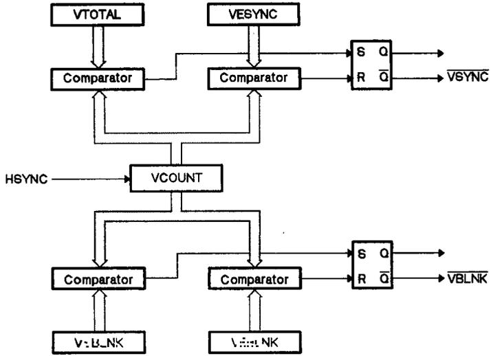
Figure 9-6. Vertical Timing Logic - Equivalent Circuit
