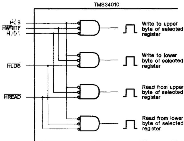
Figure 10-1. Equivalent Circuit of Host Interface Control Signals
