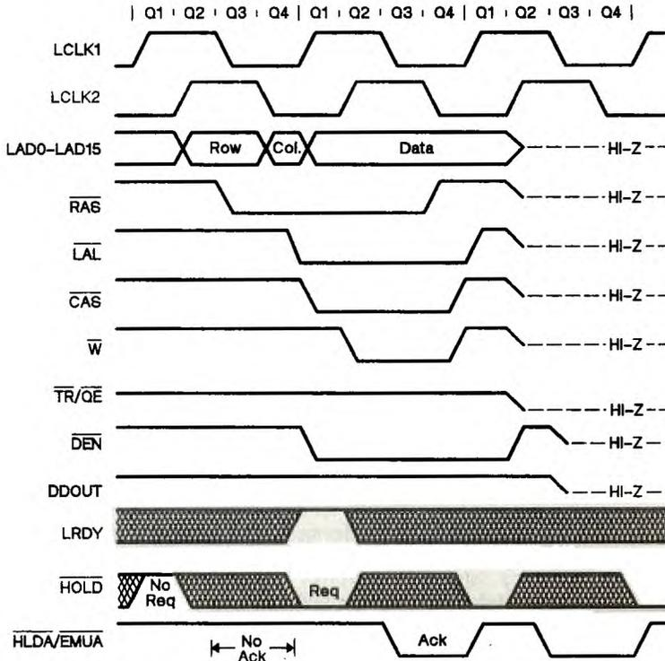
**Figure 11-15. TMS34010 Releases Control of Local Bus**
