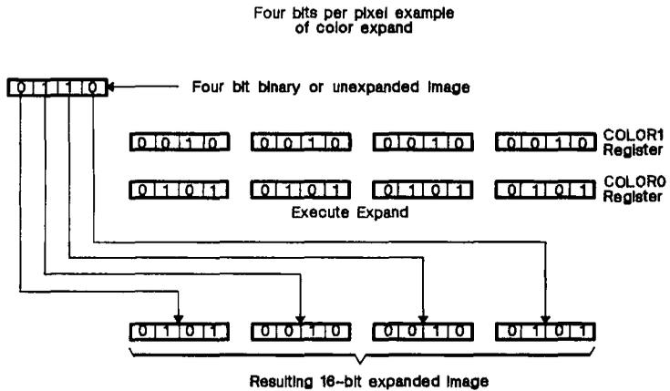
Figure 7-1. Color-Expand Operation
