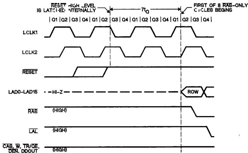
Figure 11-17. Local Bus Timing Following Reset
