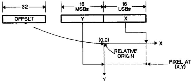
Figure 4-9. Pixel Addressing in Terms of XY Coordinates
