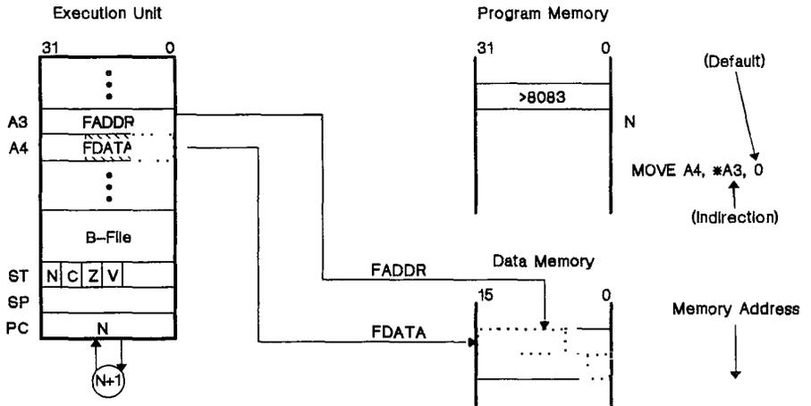
Figure 12-4. Register Indirect Addressing Mode
