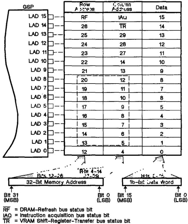
Figure 11-1. Triple Multiplexing of Addresses and Data
