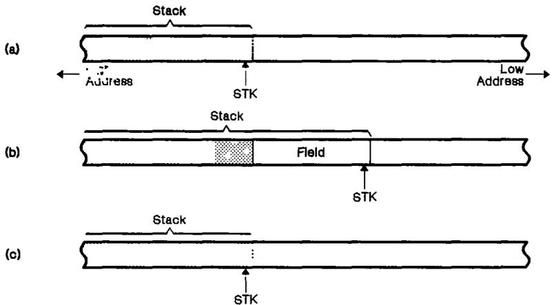
Figure 3-6. Auxiliary Stack Grows toward Lower Addresses
