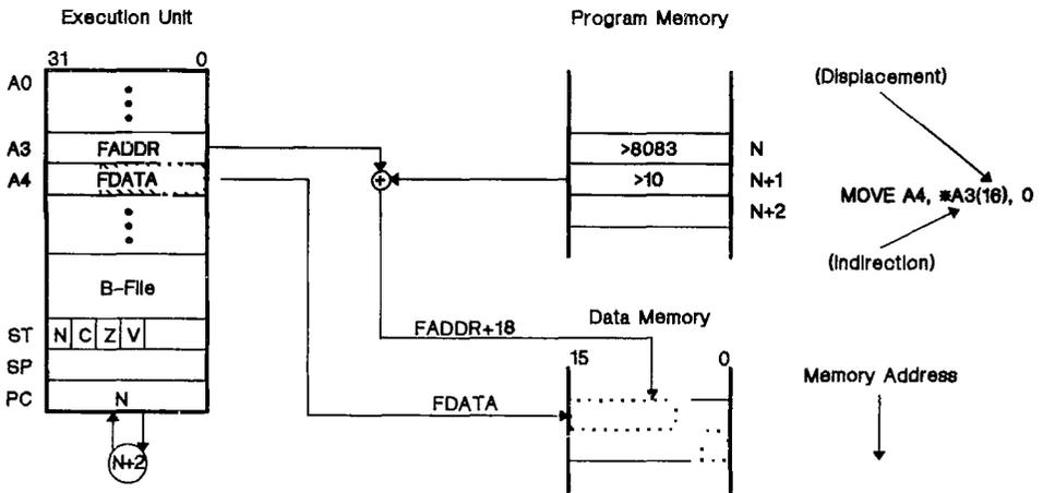
Figure 12-5. Register Indirect with Displacement Addressing Mode
