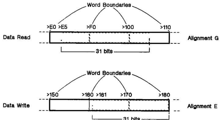
Figure 13-2. MOVE Timing Example
