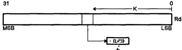
**Description** BTST tests the specified destination register bit, K, and sets status bit Z accordingly. The K value must be an absolute expression that evaluates to a value in the range 0 to 31; if the value specified is greater than 31, the assembler issues a warning and truncates the K operand value to the five LSBs. The specified bit number is 1's complemented by the assembler before it is inserted into the K field of the opcode.
