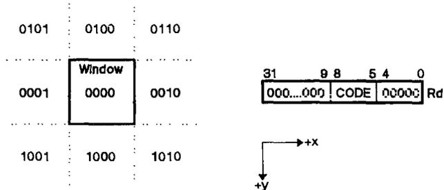
Note that the five LSBs of the destination register are set to 0 so that Rd can be used as an index into a table of 32-bit addresses.
