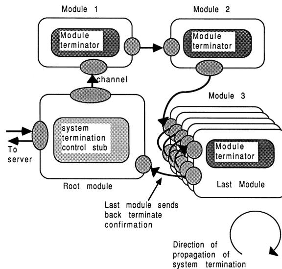
Figure 11: A system termination example
