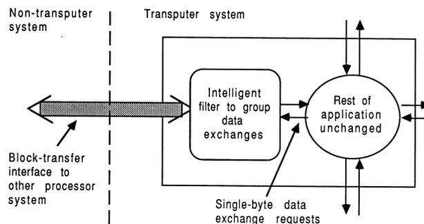
Figure 16: Using a filter to block-up data exchange requests
