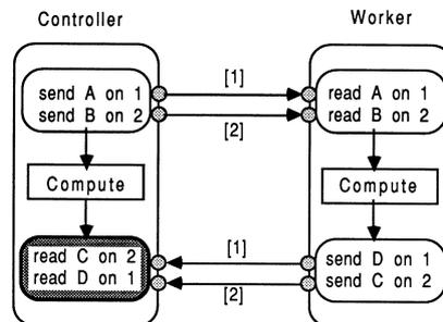
Figure 7: Deadlock due to incorrect channel ordering
