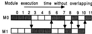
Figure 8: Module execution pattern using stubs
