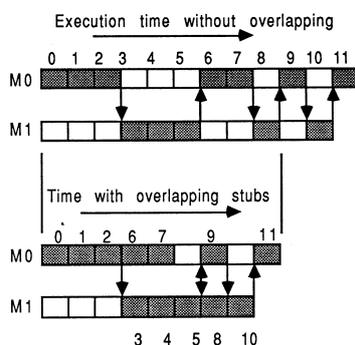
Figure 13: Overlapping execution using two stubs per module
