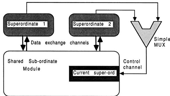
Figure 12: Sharing a common sub-ordinate module
