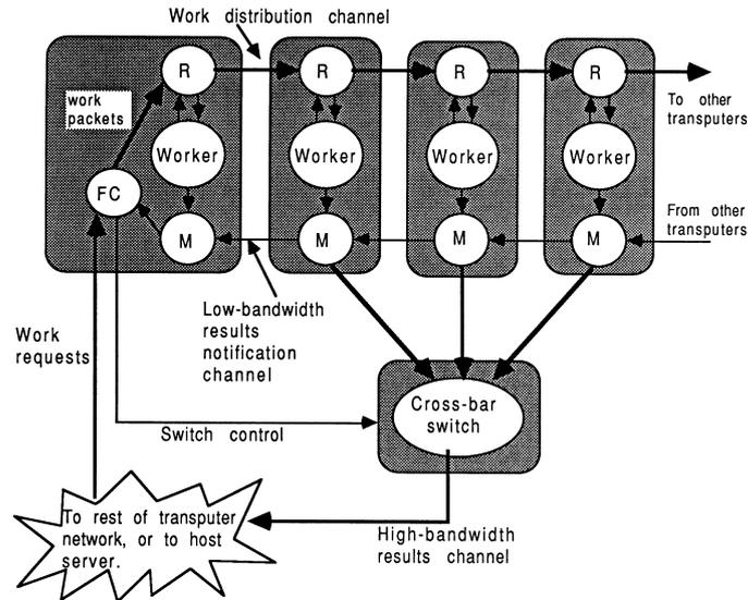
Figure 19: A dynamically re-configurable farm
