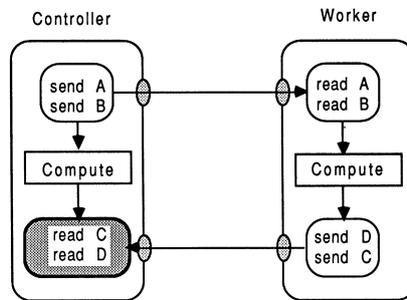
Figure 6: Incorrect message ordering on a single channel
