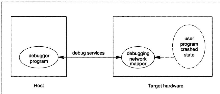
Figure 2.2 Post-mortem debugging system
