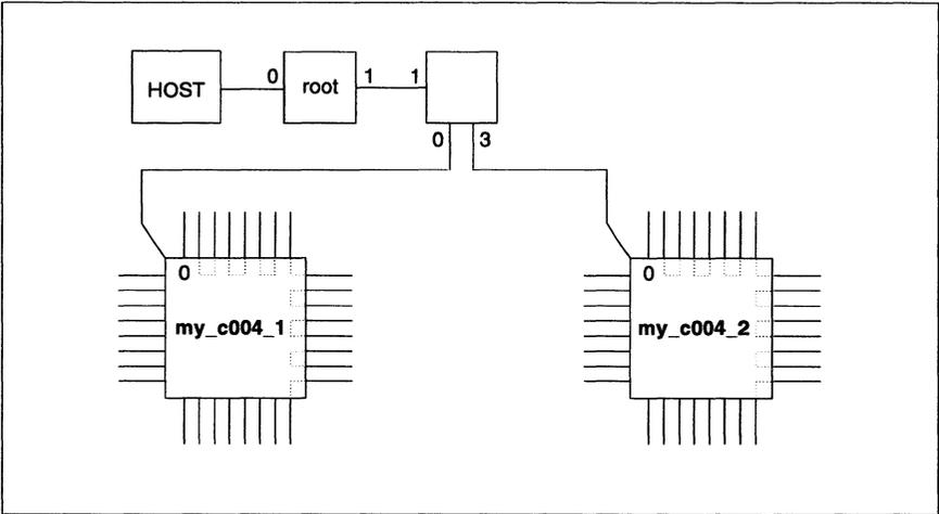
Figure 7.5 Example link switch connections
