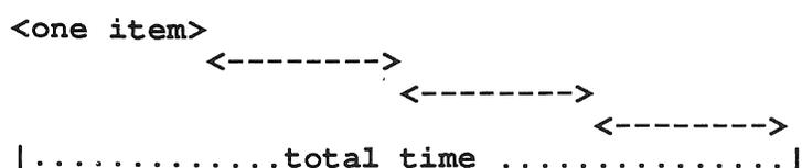
**Aside:** The time savings can be dramatic; in principle the time to process *n* numbers using a pipeline can be better than *n* times faster than a single processor, because by using smaller local memories, the memory fetch time can be reduced (cf. the car workers have less far to fetch the components). But don't forget that
