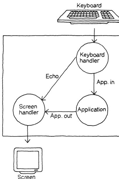
In occam, each task is represented by a process, and each connection by a channel. The processes communicate by sending messages via the channels. A process can be constructed from smaller processes. Indeed this collection of processes is itself a process in occam, and the system as described could be part of some larger system.
