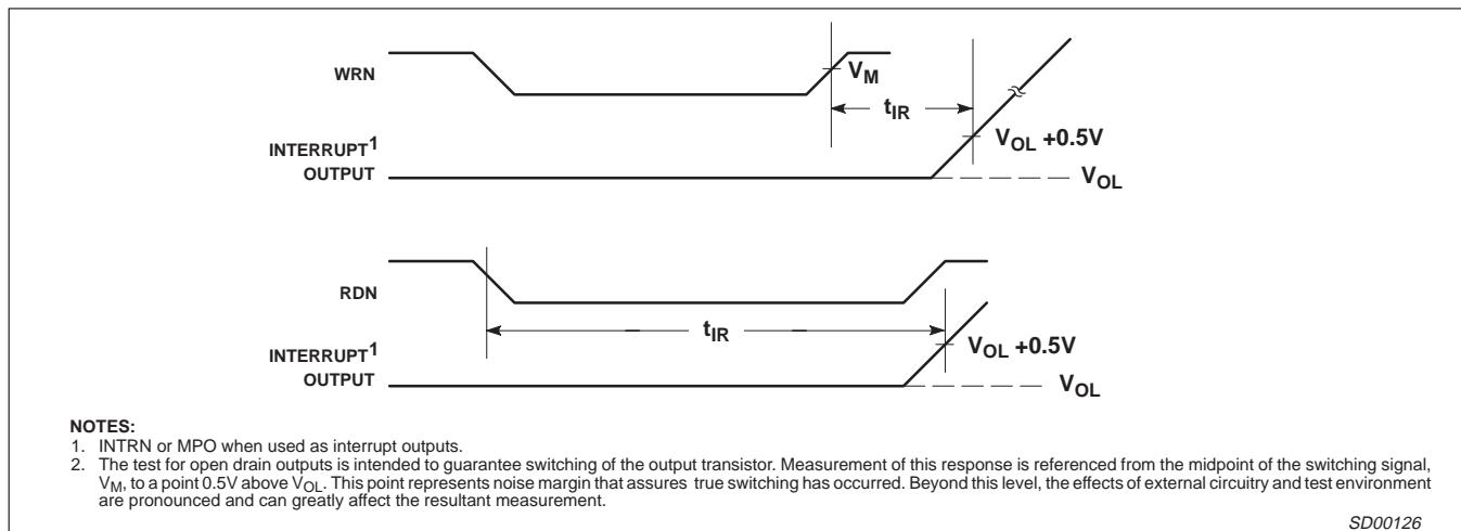
Figure 6. Interrupt Timing
