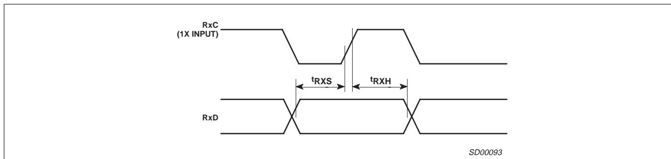
Figure 9. Receive Timing
