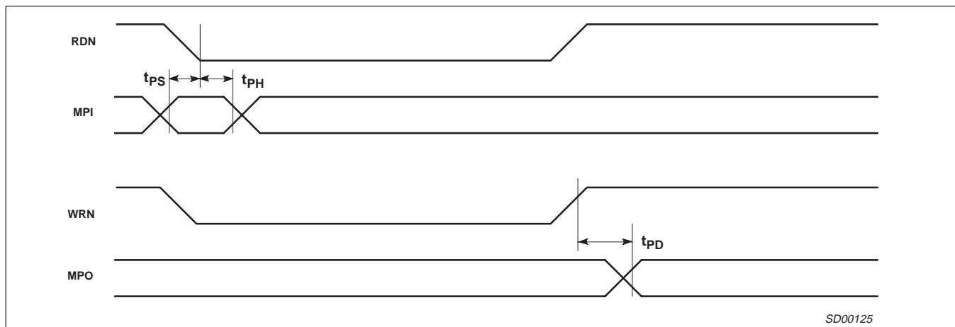
Figure 5. I/O Timing
