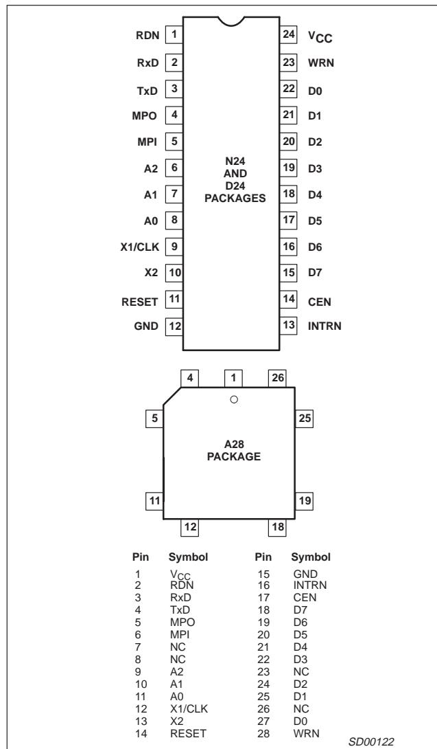
Figure 1. Pin Configurations
