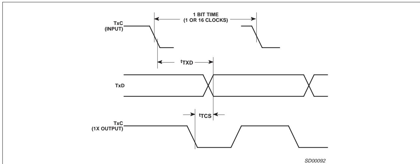
Figure 8. Transmit Timing
