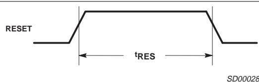
Figure 3. Reset Timing
