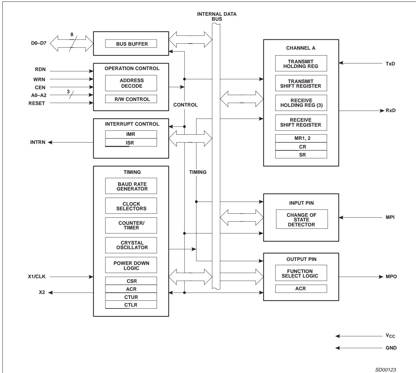
Figure 2. Block Diagram
