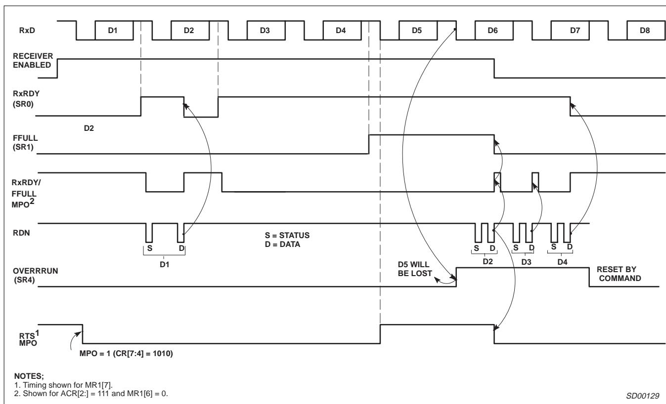
Figure 11. Receiver Timing
