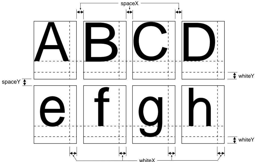
**Figure C.4 DEFAULT CELL SPACING**
