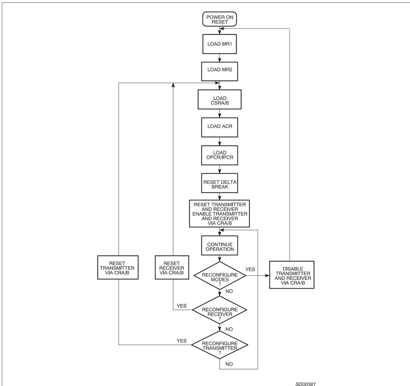
Figure 2. Asynchronous Initialization
