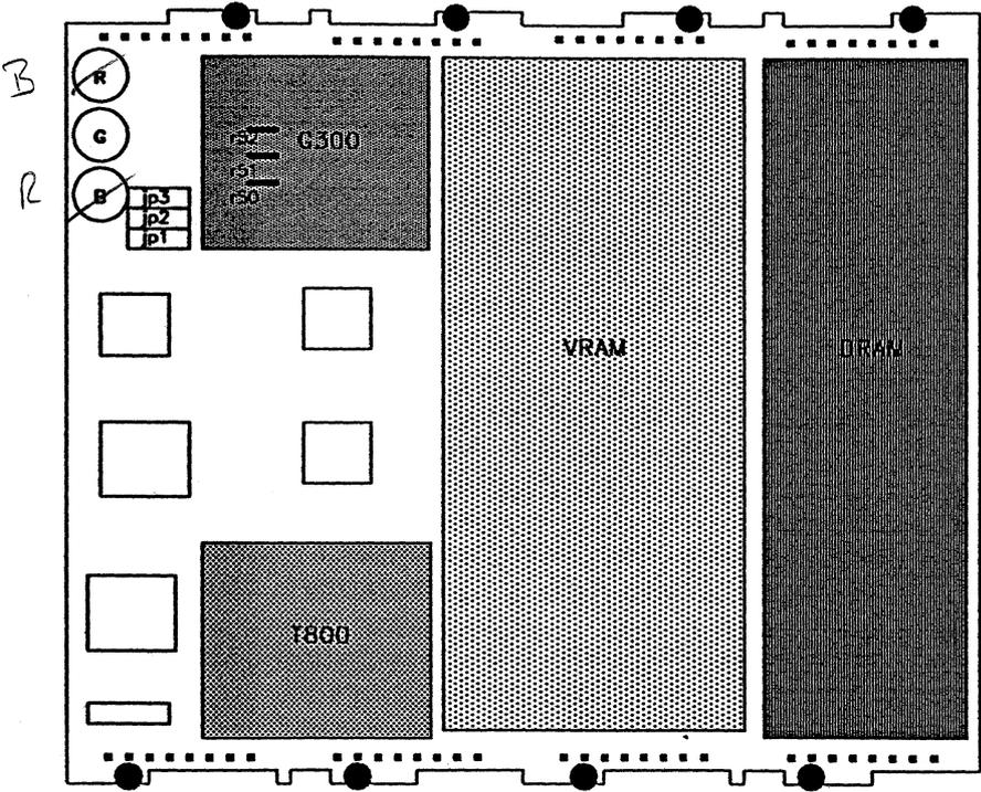
R51,R52,R53 are actually on the reverse side of the pcb under the G300
