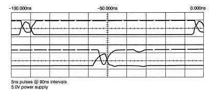
Figure 9: Isolated 5ns pulses, AT&T 41M series, 10m x 30AWG
