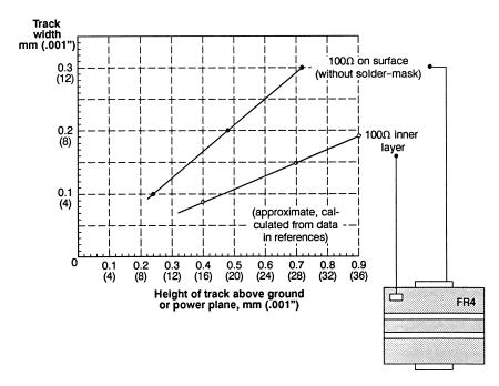
Figure 1: Approximate PCB transmission line impedance for FR4 laminate
