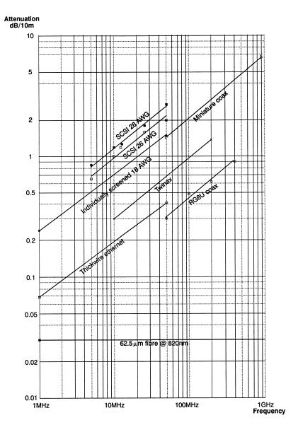
Figure 2: Cable attenuation against frequency for a variety of cables
