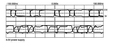
Figure 10: HP1414 LED, 2416 receiver, 100m of  $62.5\mu$  fibre
