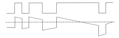
Figure 7: Effect of excessive run length
