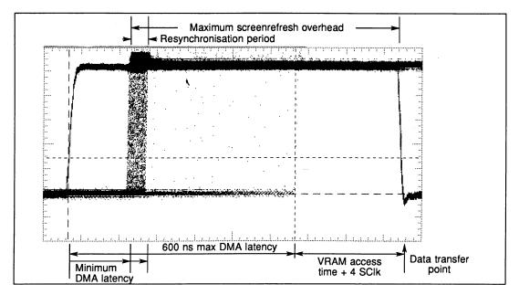
Figure 3.11 Measured DMA latency
