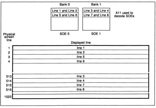
Figure 3.15 Effect of untransposed addresses on display
