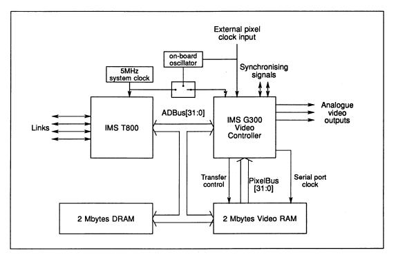
Figure 3.1 IMS G300 TRAM block diagram
