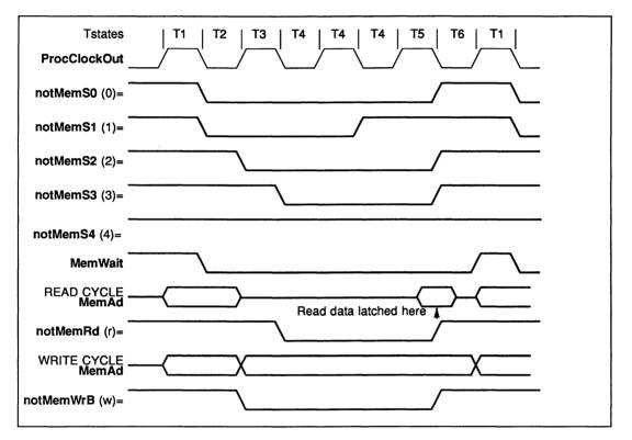
Figure A.2 Timing for basic memory cycle
