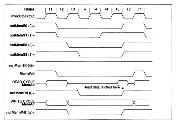
Figure 3.3 Timing for basic memory cycle
