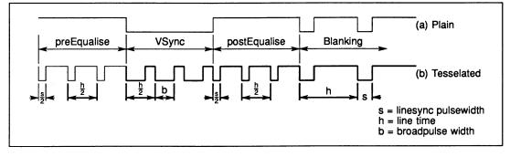
Figure 3.18 Composite sync frame flyback waveforms
