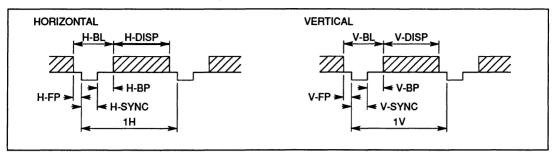
Figure A.1 Hitachi HM-4219/4119 timing
