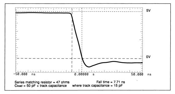
Figure 3.23 Optimally damped response
