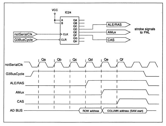
Figure 3.8 Memory strobe generation for G300 VRAM interface using a shift register
