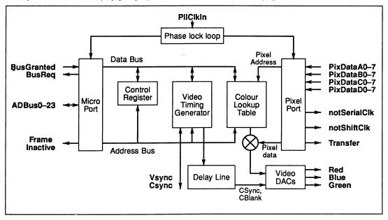
Figure 2.1 IMS G300 Block Diagram
