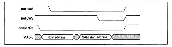
Figure 3.5 VRAM transfer timing
