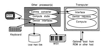
Figure 15: After the mixed-processor porting
