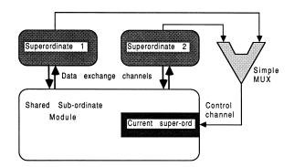
Figure 12: Sharing a common sub-ordinate module
