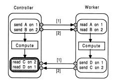
Figure 7: Deadlock due to incorrect channel ordering
