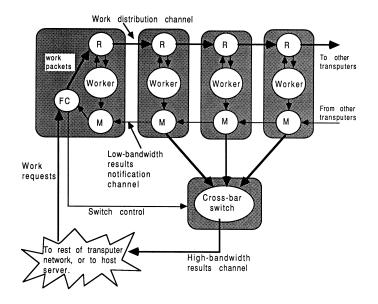
Figure 19: A dynamically re-configurable farm
