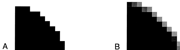
Figure 8: Magnified object silhouette A) without and B) with anti-aliasing
