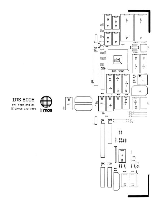
Figure 20: IMS B005 component ident
