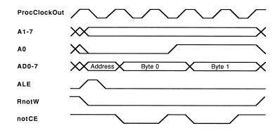
Figure 4: M212 memory timing write
