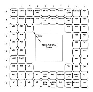
Figure 21: IMS M212 pinout
