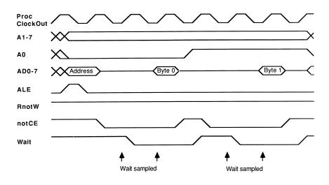
will be extended if the wait input is high. When the wait input is sampled low, the cycle will continue.
