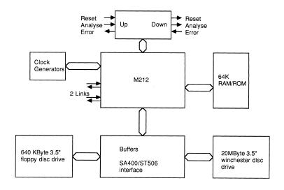
Figure 2: IMS B005 block diagram
