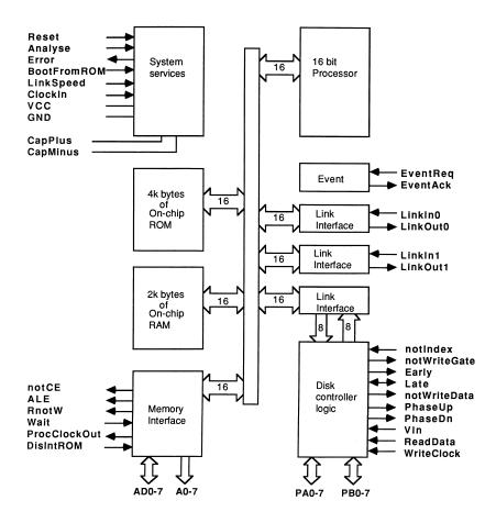
Figure 1: IMS M212 block diagram
