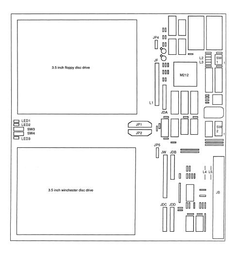
Figure 17: IMS B005 component layout
