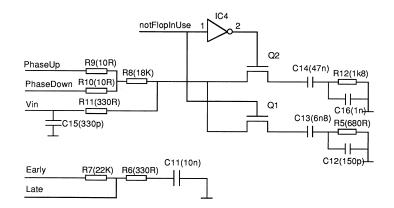
Figure 9: Filter components
