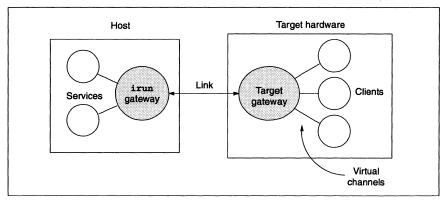
Figure 1.1 A simple software host-target interface
