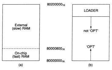
Figure 6.5 Memory Allocation in a 2MB, T414 System
