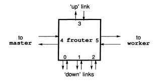
The **frouter** task is used by the flood-filling configurer as the standard task which resides on each node of a flood-filled network and manages the flow of work packets and responses through the network.
