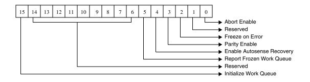
Figure 5-57. Work Queue Options For Initialize Work Queue Command
