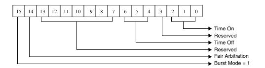
Figure 5-41. Time On/Time Off Fair Arbitration Mode Enabled
