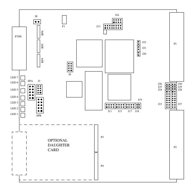
*NOTE:* P8 is a 68-pin micro D ''P'' connector P7 is a 50-pin ribbon ''A'' connector
