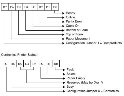
Figure 3-15. Printer Status Register
