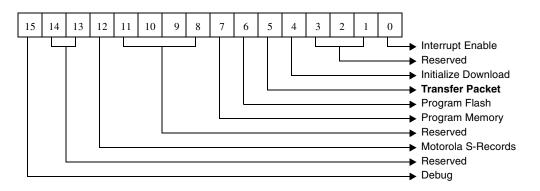
Figure 6-16. Command Options For DownLoad Firmware Command (Bit 5).
