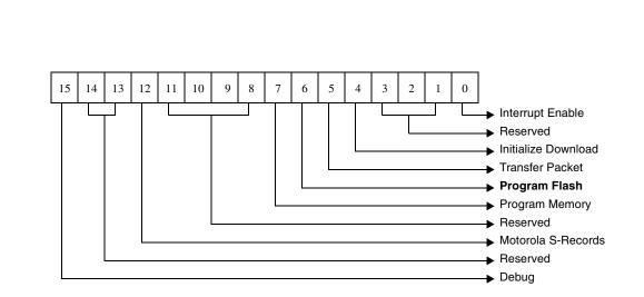
Figure 6-17. Command Options For Download Firmware Command (Bit 6)
