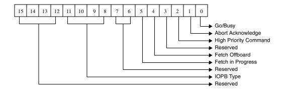
Figure 3-7. Queue Entry Control Register (QECR)
