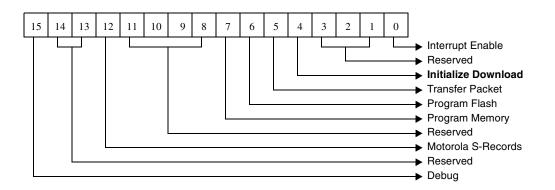
Figure 6-15. Command Options For Download Firmware Command (Bit 4).
