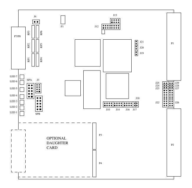
NOTE: RP7 and RP9 (not pictured) are not SCSI Terminators. Do not remove. P8 is a 68-pin micro D "P" connector P7 is a 50-pin ribbon "A" connector
