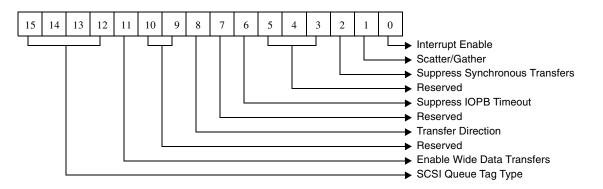
Figure 5-2. Command Options For SCSI Pass-Through Command
