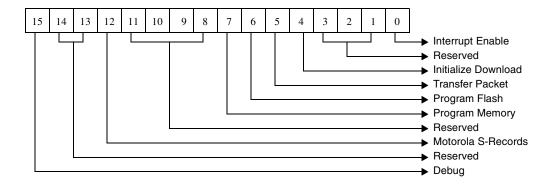
Figure 5-134. Command Options For Download Firmware Command
