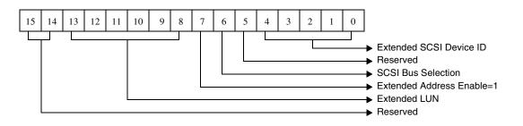
Figure 5-131. Extended Unit Address For Issue Abort Message Command
