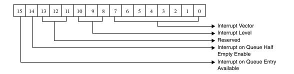
Figure 3-4. Interrupt On Queue Available Register (IQAR)
