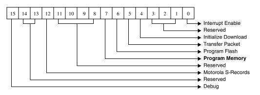
Figure 6-18. Command Options For Download Firmware Command (Bit 6).
