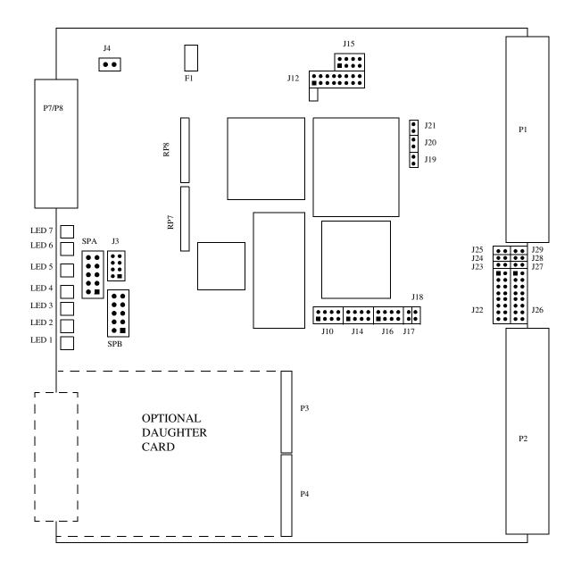
P8 is a 68-pin micro D "P" connector P7 is a 50-pin ribbon "A" connector
