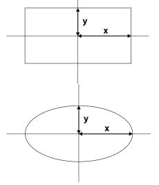
If the ellipse mode is selected (Vmode = 1), the value stored in Vx represents 1/2 of the length of the horizontal axis of the ellipse (expressed in pixels), and the value stored in Vy represents 1/2 of the length of the vertical axis of the ellipse (expressed in pixels) to be used for the pen point.
