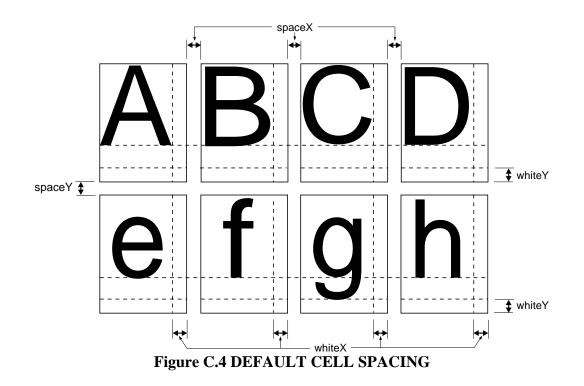
The shape of an individual character is defined by a bit-map array of the same dimensions as the character cell (fontX• fontY). Each bit in the array corresponds to a pixel within the character cell. The pixels within the character cell can be numbered from left-to-right, top-to-bottom, contiguously throughout the cell—this corresponds to the numbering of the bits in the bit-map array in order of their bit-addresses. Successive character cells are packed contiguously in the font shape data.
