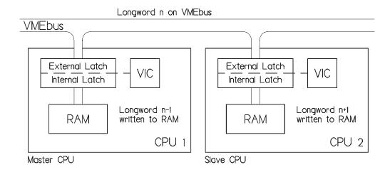
Figure 4. Block Transfer Read Cycle
