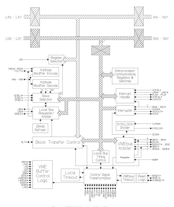
Figure 1. VIC068A Functional Block Diagram
