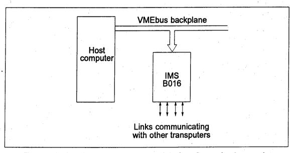
Figure 1.2 The IMS B016 used as an interface from a host computer
