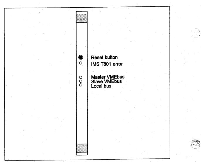
Figure 2.4 Front panel showing LEDs
