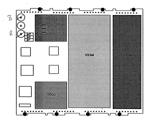
R51,R52,R53 are actually on the reverse side of the pcb under the G300
