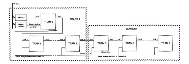
Figure 6: Two Cascaded Boards
