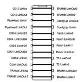
Figure 15: 24-way Patch Header Connections
