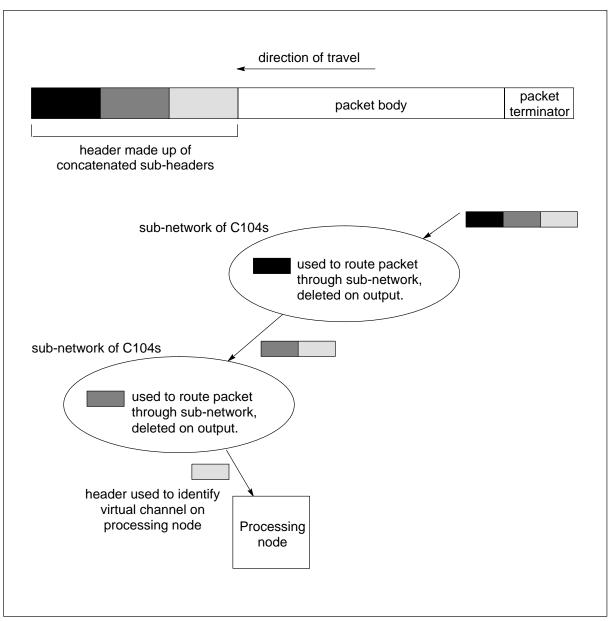
Figure 3.8 Hierarchical composition of networks using header deletion
