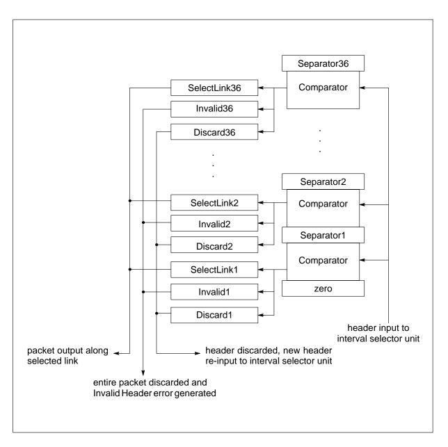
Figure 3.6 Interval selector registers
