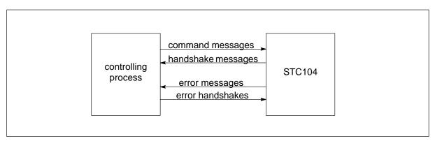
Figure 5.1 Communication between the controlling process and the STC104
