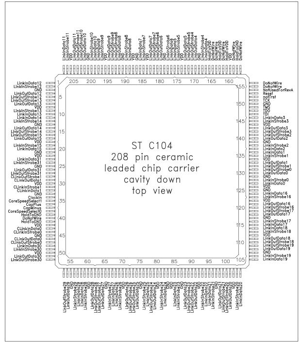
Figure 13.1 STC104 208 pin CLCC cavity-down package pinout
