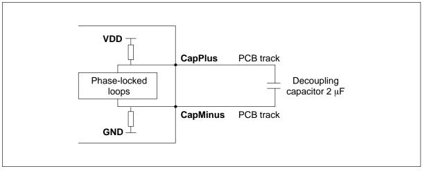
Figure 9.1 Recommended PLL decoupling
