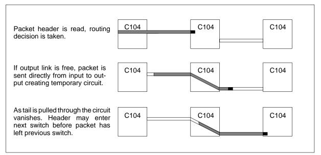
Figure 3.3 Wormhole routing
