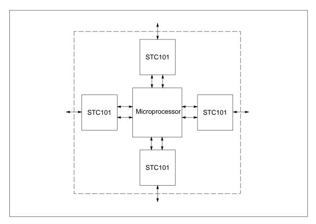
Figure 2.1 Processing node
