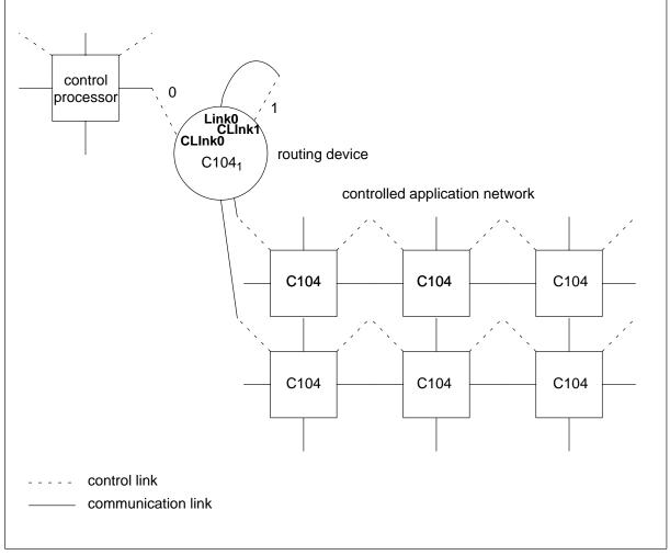
Figure 5.7 An STC104 providing fan-out.
