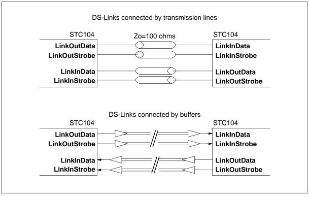
Figure 6.2 DS-Link connections
