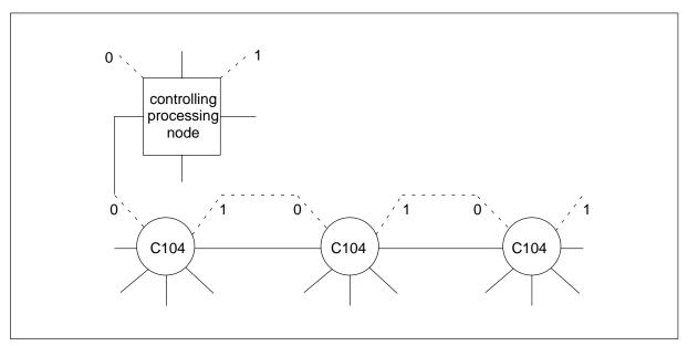
Figure 5.2 A daisy-chained control link network
