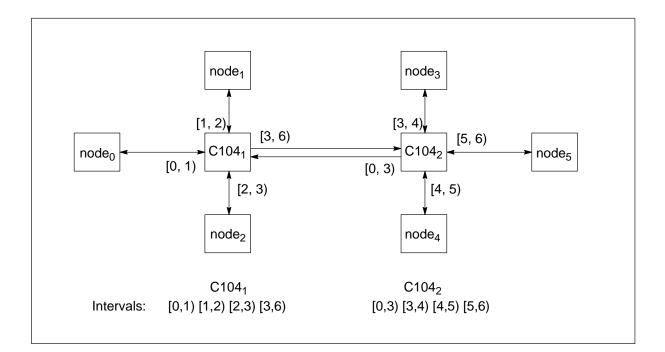
Figure 3.5 Interval routing
