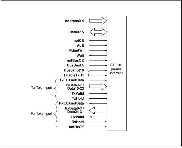
Figure 5.3 16-bit processor interface with token interfaces
