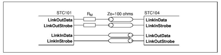
Figure 15.9 DS-Links connected by transmission lines
