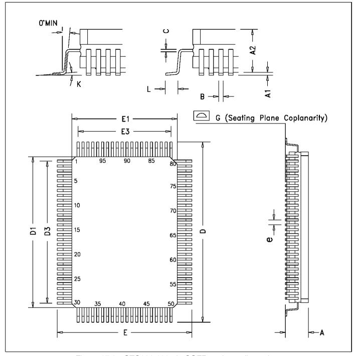
Figure 17.2 STC101 100 pin CQFP package dimensions
