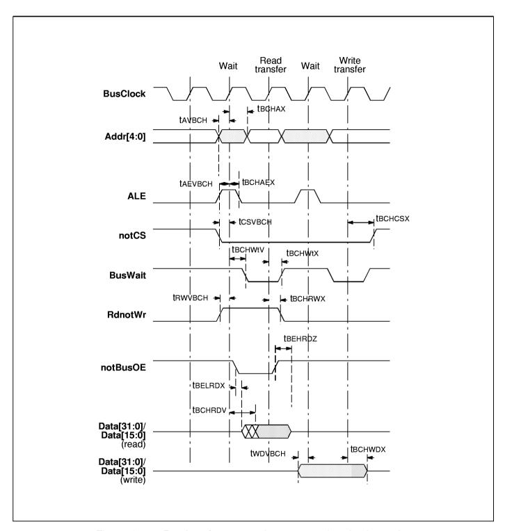
Figure 15.6 Bus interface – synchronous read and write cycles
