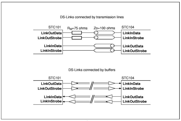
Figure 9.2 DS-Link connections
