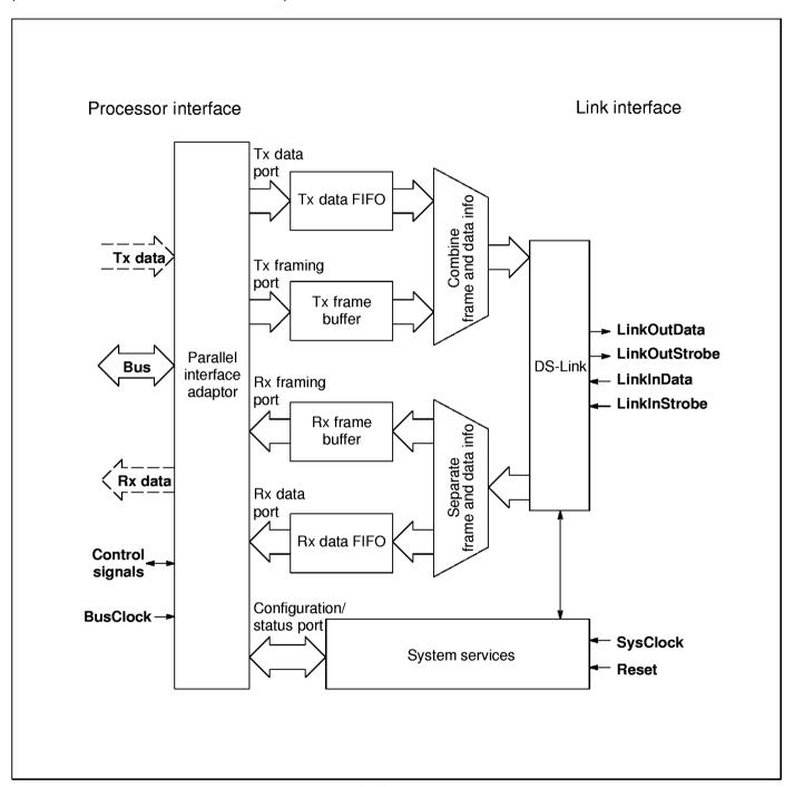
Figure 3.1 STC101 block diagram
