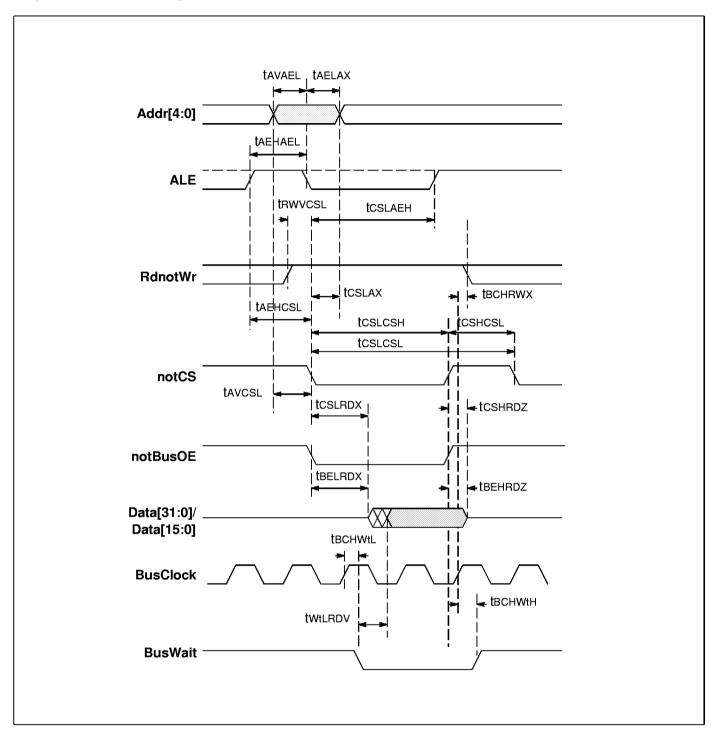
Figure 15.4 Bus interface – asynchronous read cycle
