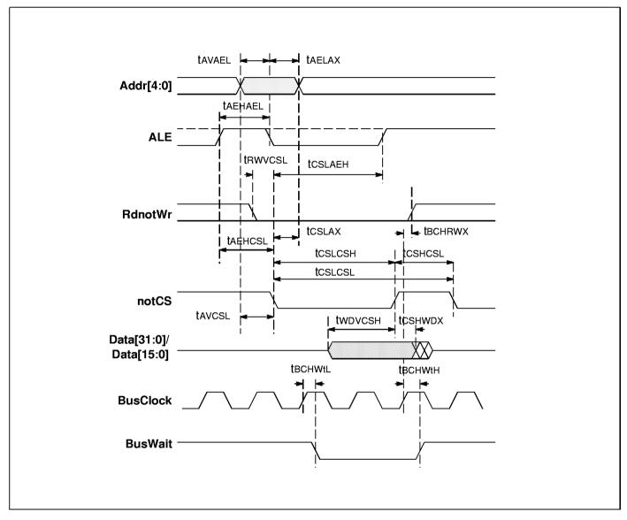
Figure 15.5 Bus interface – asynchronous write cycle
