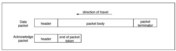
Figure 2.1 Structure of a packet on DS-Links
