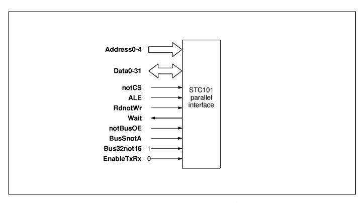
Figure 5.2 32-bit processor interface
