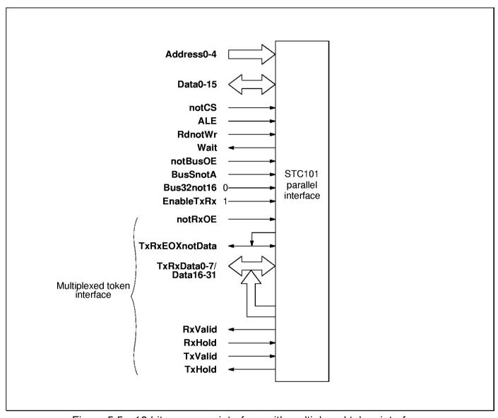
Figure 5.5 16-bit processor interface with multiplexed token interfaces
