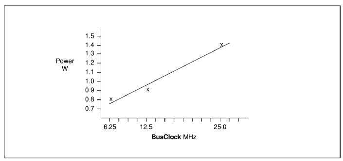
Figure 16.1 Power dissipation vs **BusClock** frequency
