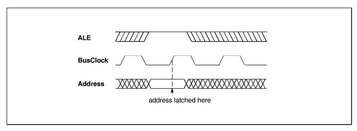
Figure 15.3 Address latching in synchronous mode
