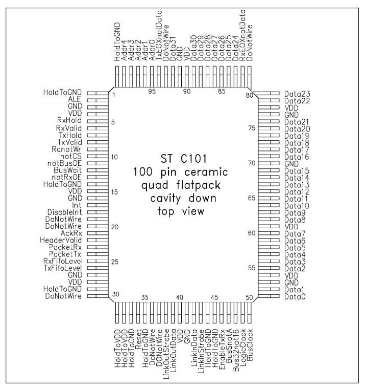
Figure 17.1 STC101 100 pin CQFP package pinout
