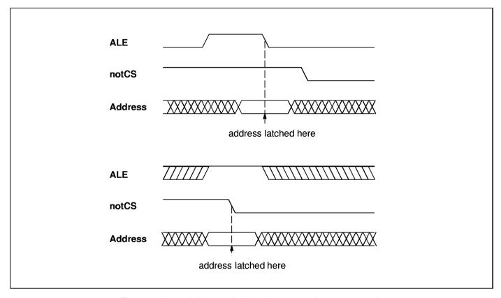
Figure 15.2 Address latching in asynchronous mode
