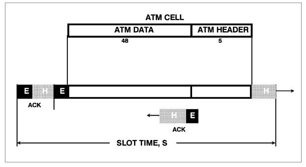
Figure 10.30 Bidirectional Single–Packet ATM–DS-Link Mapping
