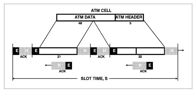
Figure 10.31 Bidirectional Double–Packet ATM–DS-Link Mappings
