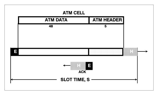
Figure 10.28 Unidirectional Single–Packet ATM–DS-Link Mapping
