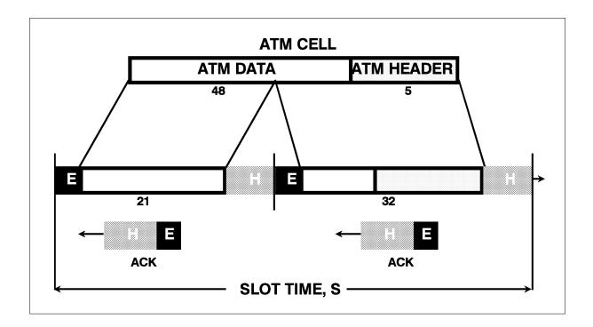
Figure 10.29 Unidirectional Double–packet ATM–DS-Link Mapping
