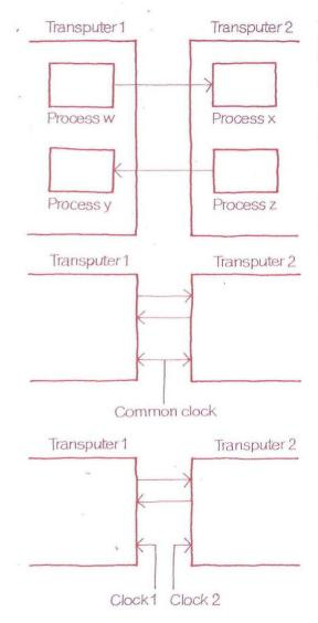
The IMS T424 has four standard INMOS links providing high speed intercommunication between transputer products, enabling a rich variety of networks to be constructed. Each link operates independently, and provides a memory to memory message (block) transfer capability between transputers.
