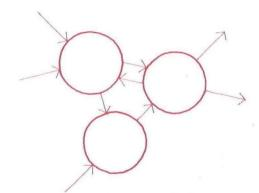
Processes can be connected together by channels to build more complex concurrent systems
