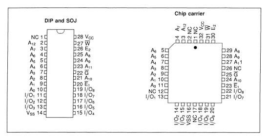
Figure 2.12 8K x 8 pin configuration
