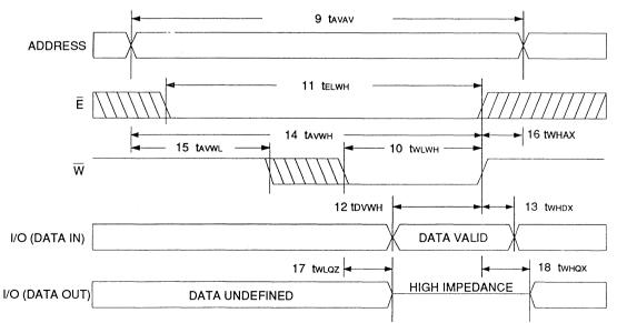
RECOMMENDED AC OPERATING CONDITIONS ( $-55^{\circ}C \le T_{A} \le 125^{\circ}C$ ) ( $V_{CC} = 5.0V \pm 10\%$ )
