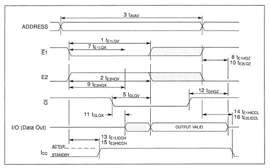
Figure 2.3 Read cycle 2<sup>c</sup>
