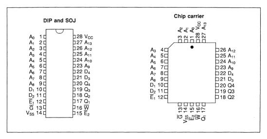
Figure 2.11 16K x 4 (with separate Inputs and Outputs) pin configuration
