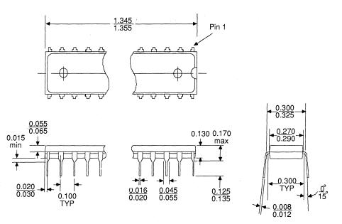
Note: All measurements are in inches. Top figure denotes minimum dimension; bottom figure denotes maximum dimension.
