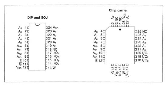
Figure 2.10 16K x 4 (with output enable) pin configuration
