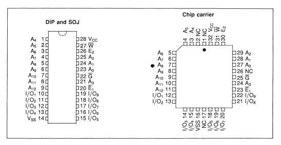
Figure 2.13 8K x 9 pin configuration
