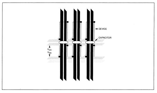
Figure 2.6 Grid showing decoupling capacitors
