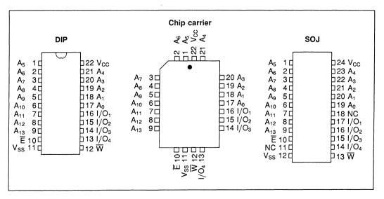
Figure 2.9 16K x 4 pin configuration
