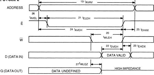
the memory becomes active. The data from the memory will be the same as the input data unless the input data or address changes.
