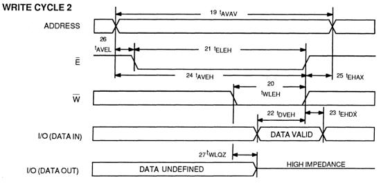
WRITE CYCLE 2 waveform shows a write cycle terminated by  $\overline{E}$  going high. Data set-up and hold times are referenced to the rising edge of  $\overline{E}$ . With  $\overline{E}$  high, the outputs remain in the high impedance state.
