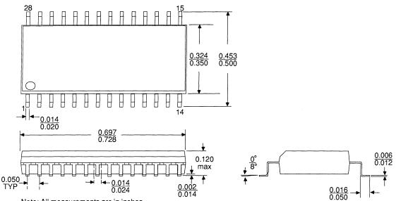
Note: All measurements are in inches. Top figure denotes minimum dimension; bottom figure denotes maximum dimension.
